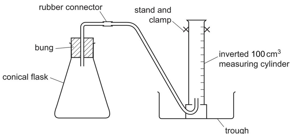
Note: The trough should be large enough to allow the measuring cylinder to be filled with water in the trough.
