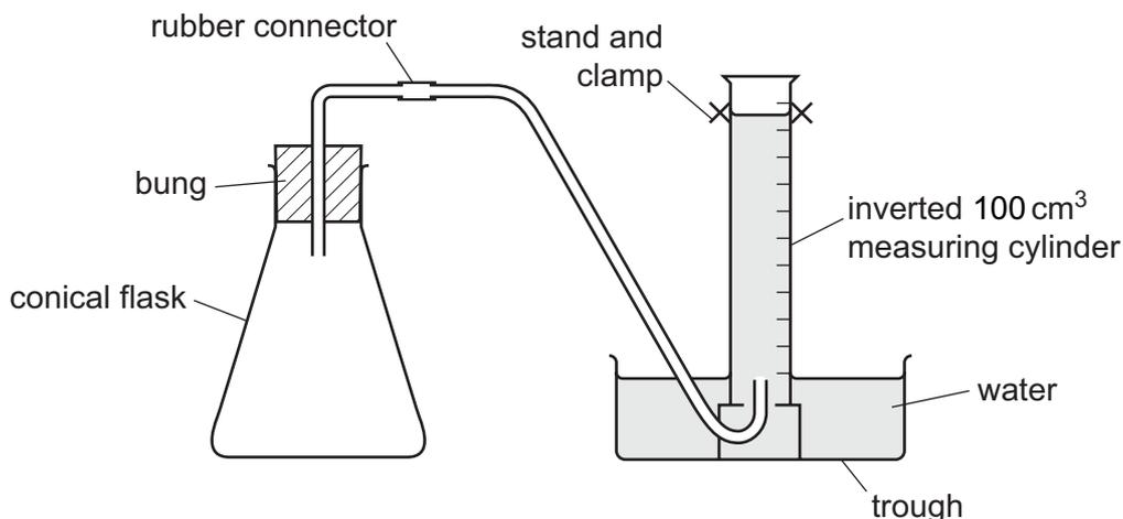
Remove the bung from the conical flask and move the measuring cylinder away from the delivery tube without letting any water run out. Twist one of the strips of magnesium to break it into four pieces and place all four pieces into the conical flask.
