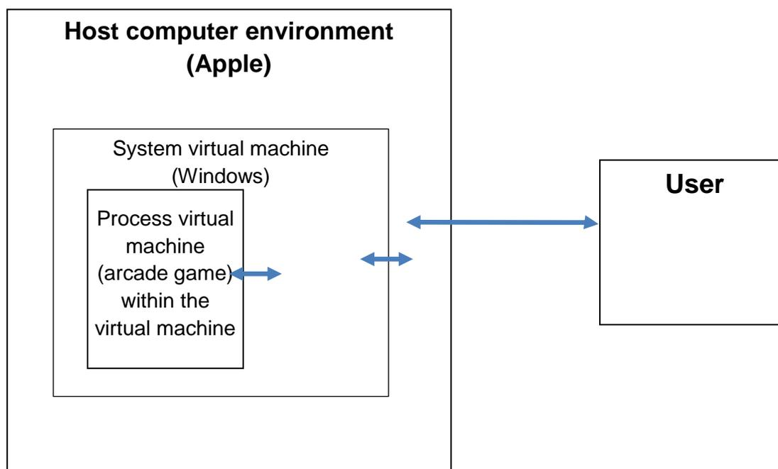
The number of virtual machines within virtual machines is limited only by the hardware's performance and available memory of the host computer.
