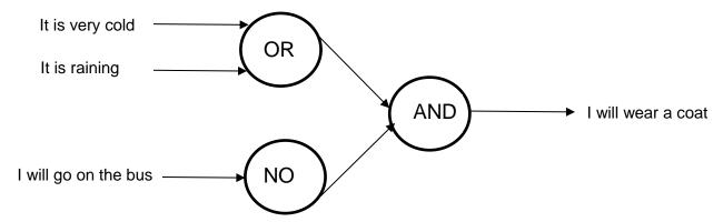
If we look at the logic of our diagram we can see that if it is very cold or it is raining and I am not going on the bus, I will wear a coat. But if I go on the bus I will not wear a coat regardless of whether it is very cold or it is raining.
