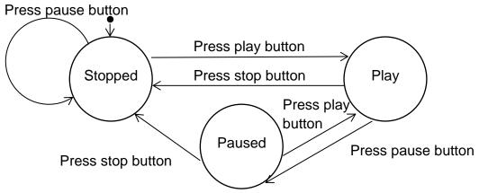
The event (press pause when state is Stopped) that does not cause any change in state is indicated by the circular arrow.
