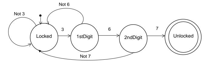
The double line around the Unlocked state indicates that lock halts in this state – this is also known as the 'accepting state'.
